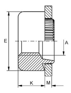
Female thread A = M2Height K = 3.0Outer diameter E = 8.0Plate thickness = 1.4 to 1.6
